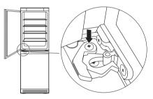
17. Place the lower door bearing with the bearing pivot in the lower left of the freezer compartment door and fasten.
